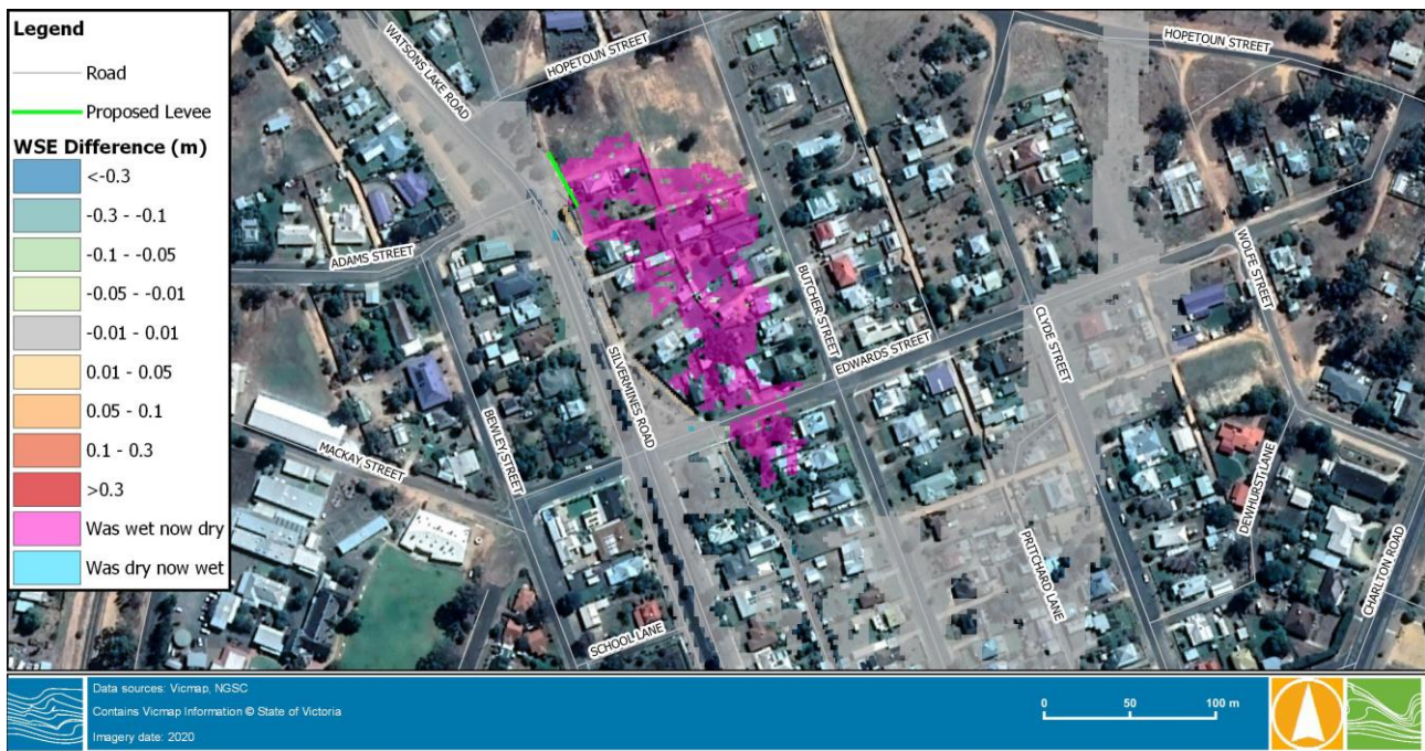
FIGURE 6-6 1% AEP WSE DIFFERENCE – WATSONS LAKE ROAD LEVEE
