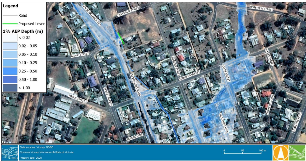
FIGURE 6-5 1% AEP DESIGN FLOOD DEPTH AT ST ARNAUD NORTH WITH LEVEE
