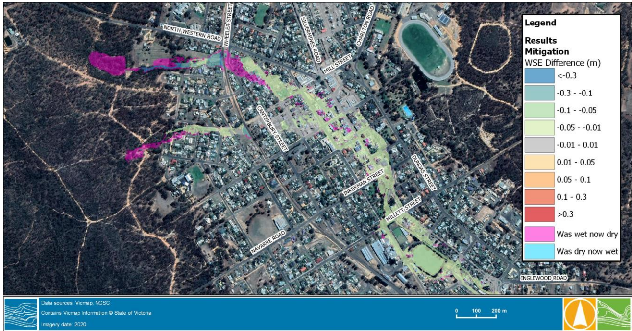
FIGURE 6-17 CHANGE IN 1% AEP, 6HR WATER LEVELS DUE TO THE REMOVAL OF FLOW CONTRIBUTION FROM THE WESTERN ST ARNAUD CATCHMENTS
