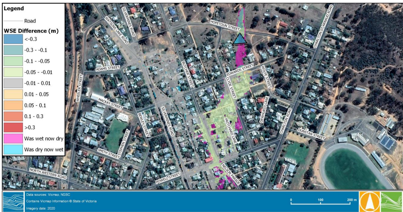
FIGURE 6-9 1% AEP WSE DIFFERENCE – GULLY DAM AT HOPETOUN STREET SOUTH
