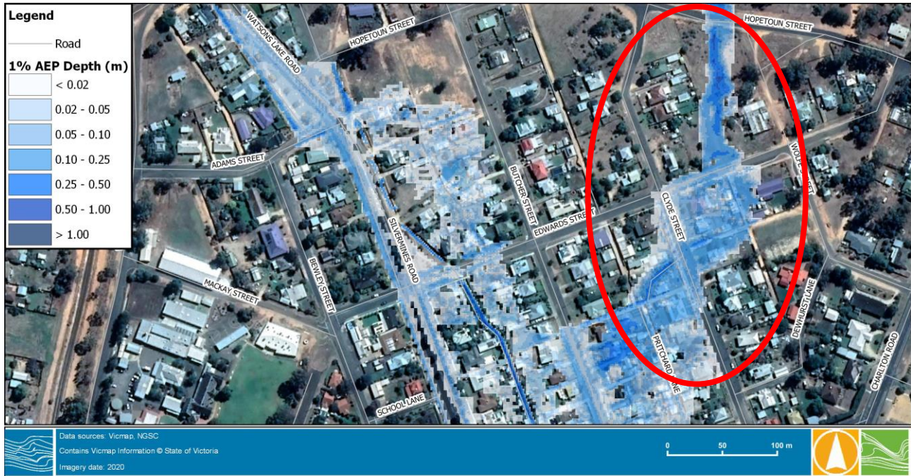
FIGURE 6-7 1% AEP DESIGN FLOOD DEPTH AT ST ARNAUD NORTH – NORTH OF EDWARDS STREET
