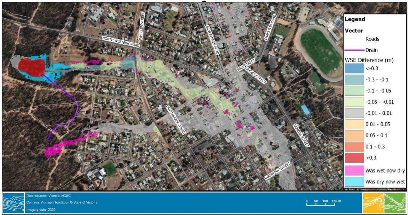
FIGURE 6-13 1% AEP WSE DIFFERENCE – REINSTATEMENT OF DAM WALL WITH DIVERTING DRAIN
